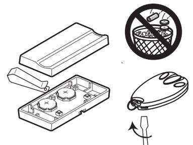
To replace cover, snap shut along both sides. The lithium batteries should produce power for up to 5 years. To replace batteries, use a coin, the visor clip or screwdriver blade to pry open the case, as shown ("Open" location is stamped on back.)
